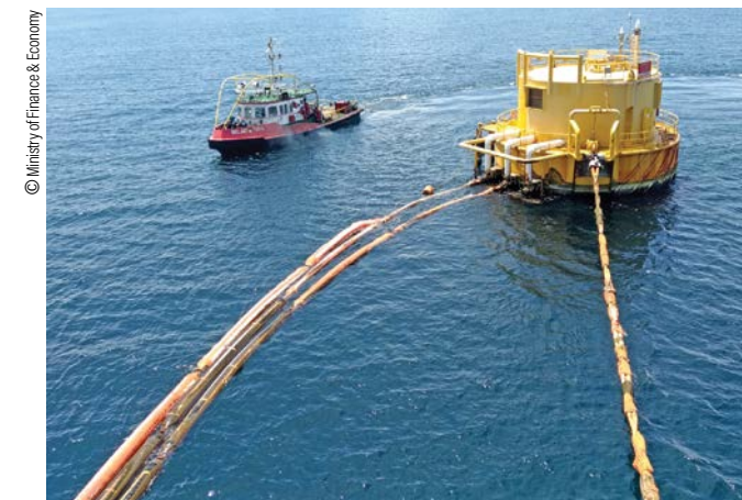
Brunei Methanol Company's export hub offers single point mooring for large ships
